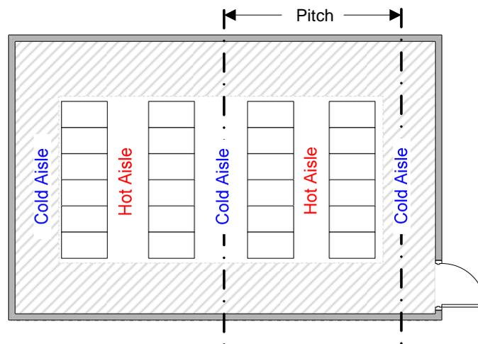
**Figure 6** shows the four standard pitches used in data center floor layouts. Each pitch is defined by a number of tiles, where a tile is 2 ft (600 mm) wide. Note that in all four pitches, the equipment racks are aligned to tiles in the cold aisles. This is because, in a raised-floor environment with perimeter-based cooling, full perforated tiles are needed in the cold-aisles for air delivery.
