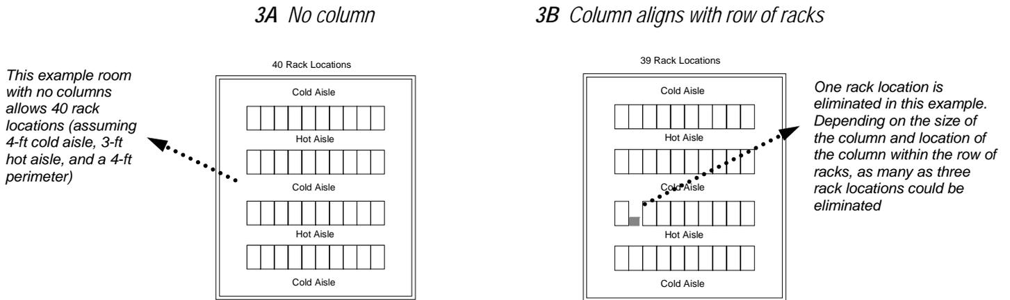
Figure 4 – Sample impact of columns on number of rack locations when column aligns with aisle
