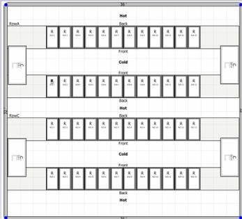
The diagram shows a top-down view of a data center aisle. It features two rows of server racks. Each row has a central 'Cold' aisle and two side 'Hot' aisles. The racks are labeled 'Front' and 'Back'. The layout illustrates how cold air is contained within the central aisle in a row-based cooling system.
