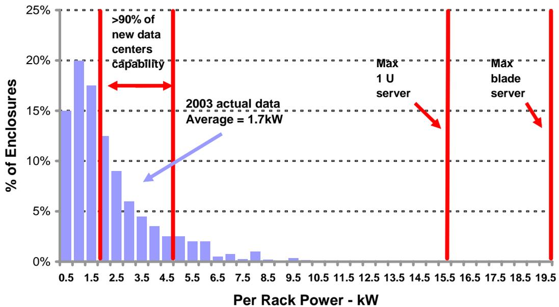
Superimposed on the actual per-enclosure power consumption values in **Figure 2**, are a number of reference lines. The first pair of reference lines indicates the range of average power densities that new data centers are designed for, based on a survey of consulting engineers.
