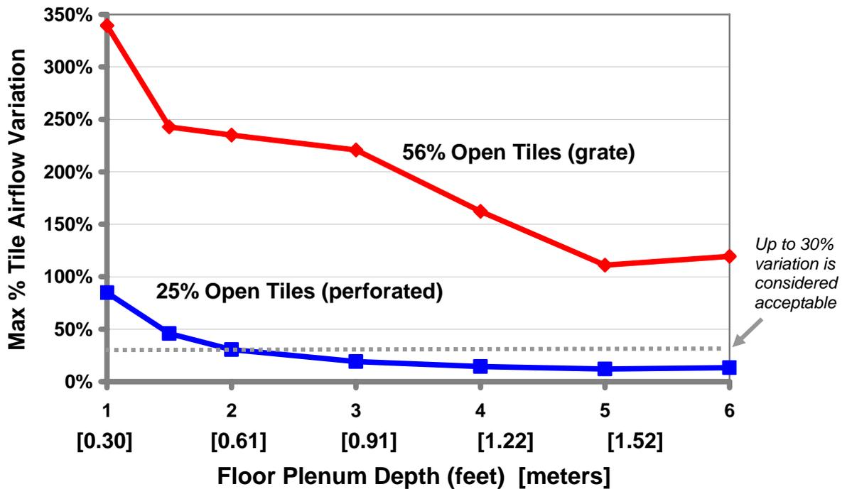
Even when an “extreme” cooling design is implemented, **Figure 3** indicates that 3 to 4 grate-type tiles would be needed to cool a hypothetical 18 kW rack enclosure. However, the typical data center layout provides only 1 floor tile per rack enclosure. When this data is combined with the airflow variation data of **Figure 4**, it suggests that **conventional data center layout with one vented tile per rack simply cannot cool racks of over approximately 6 kW per rack over a sustained area.**
