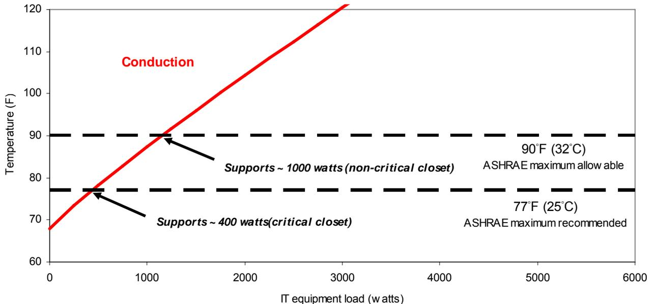
The relationship above assumes an effectively sealed 10 x 10 x 10 foot (3 x 3 x 3 meter) room with only 50 cubic feet per minute (23.6 liters per second) of air leakage, drywall construction, and all four walls opposite comfort cooled spaces at 68°F (20°C). See the **appendix** for further details and assumptions.
