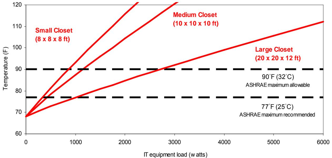
Material used for walls, ceiling, and floor will also provide a similar deviation in the relationship between temperature and load as the ability to transfer heat differs from one material to the next. If we substitute the gypsum board walls and acoustic tile ceiling in the example above for 4 inch (10 cm) concrete block walls
