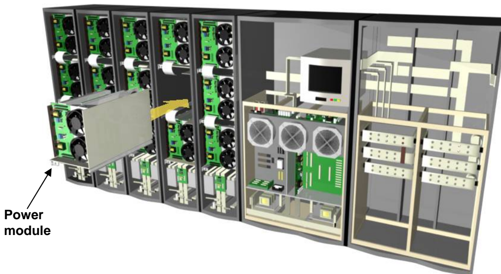
Figure 11 – A modular, scalable UPS system
