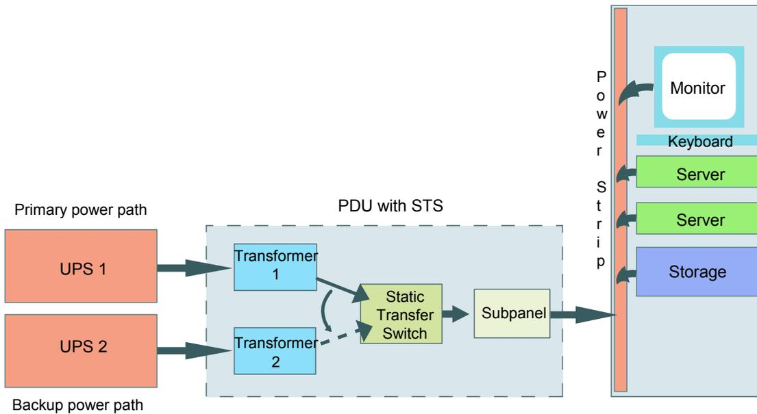
**Figures 3 and 4** are an improvement over the data center configurations shown in **Figures 1 and 2**, but they still do not offer full redundancy to the rack. Although a redundant UPS and transformer are added, the static switch, subpanel and their associated wiring are single points of failure.
