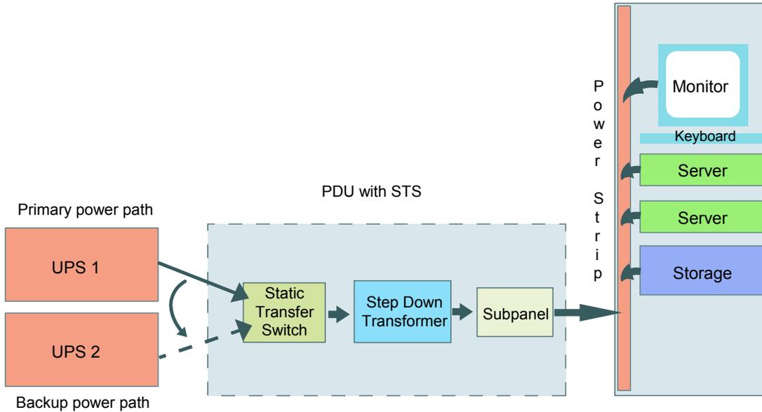
**Figure 4 – Redundancy to the load with STS (redundant transformers)**
