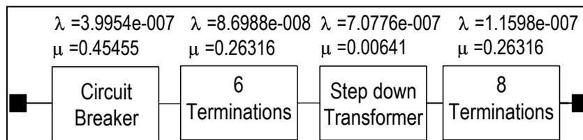
**Figure 11 – Subpanel parts**
