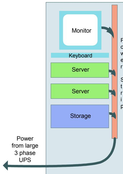
**Figure 1** shows a typical rack power distribution configuration used in small or medium size data centers and wiring closets. This configuration allows for easily moved racks with internal UPS battery backup and surge protection. In data centers where dozens or hundreds of racks are used, **Figure 2** with a large centralized UPS is a more common configuration. There is no power redundancy in the power distribution to the rack in either case.
