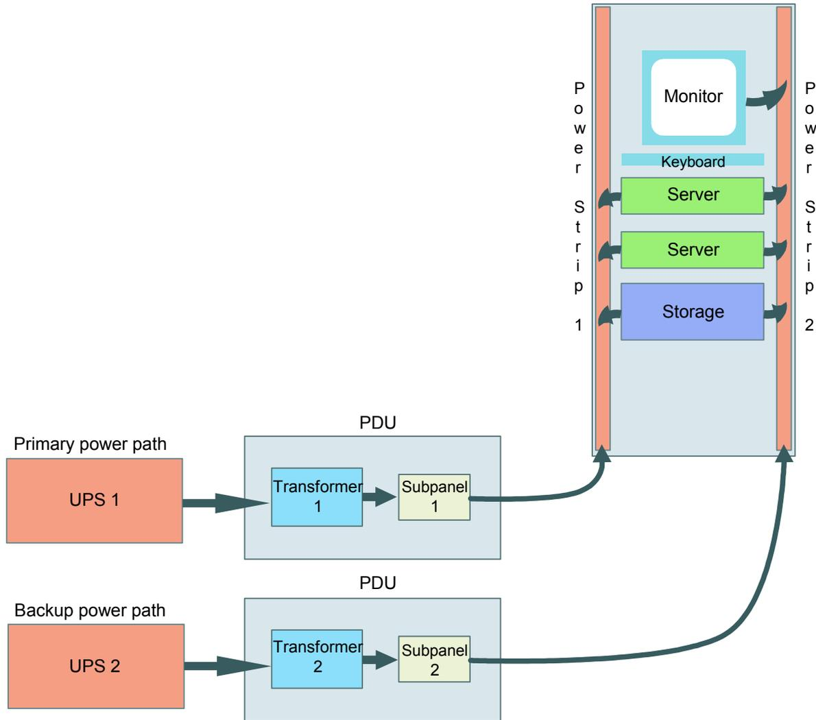
The architecture in **Figure 7** combines the architectures of **Figures 5** and **6**, and shows an alternate solution that accommodates both single and dual-corded loads. This solution employs a hybrid combination of previously reviewed designs. Full power redundancy is maintained for the dual-corded computer equipment. For the single-corded equipment, redundancy is maintained up to the Rack ATS, however, the switch and equipment power supplies are now single points of failure.
