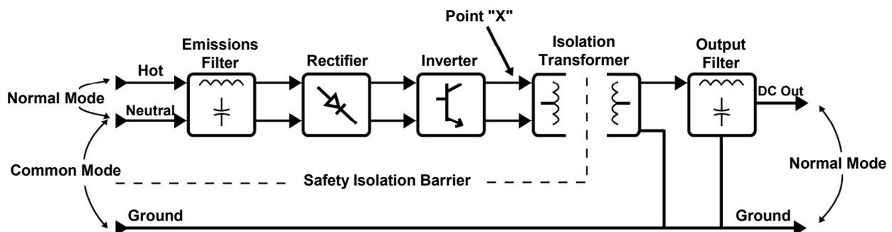
One interesting feature to note in the diagram is that there is actually no physical wire connection between the noisy power lines and the power supply output. In fact, international safety agency requirements stipulate that there must be a minimum of 1/2 cm of physical spacing between input and output. Power is transferred using the magnetic field coupling of an isolation transformer.
