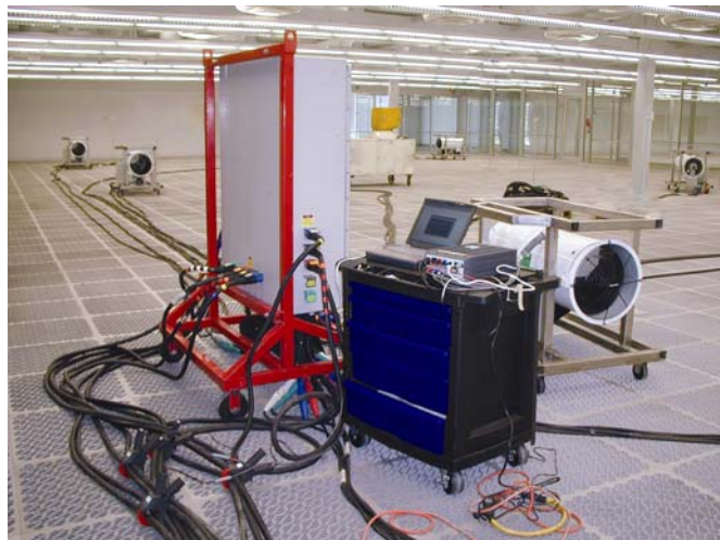
Figure 8 – Large load banks simulate computer load
