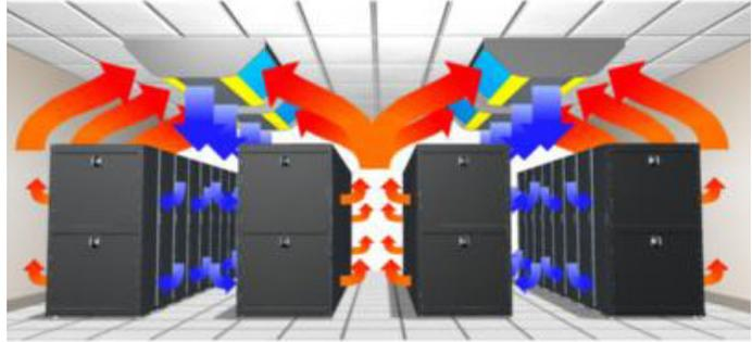
The in-row system of **Figure 2a** can also be configured as a hot-aisle containment system that extends the power density capability. This design further increases the performance predictability by eliminating any chance of air mixing.
