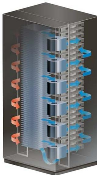
The example shows a server rack with an adjacent cooling coil/fan unit located at the side of the rack. The hot exhaust air from the servers is drawn through the cooling coils and the resulting cool air is re-circulated to the server air intakes.
